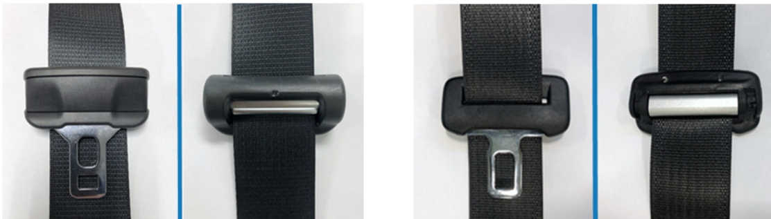
Examples of dynamic latch plates—front and back views
