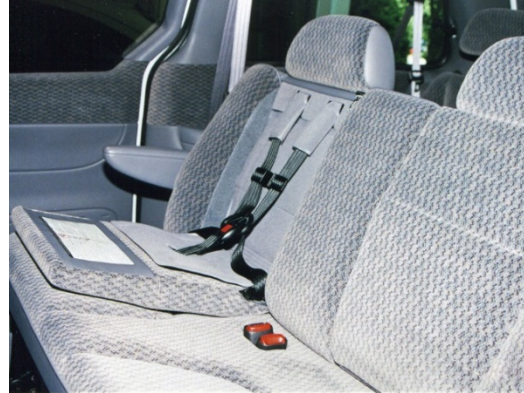
An integrated car seat is built in to the vehicle
