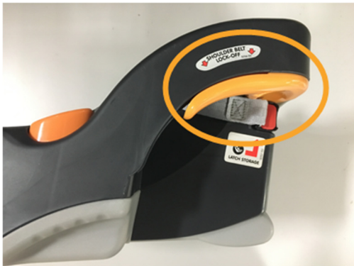
Lock-off on the side of a rear-facing only car seat base
