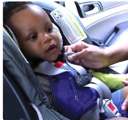
Pinch test example: harness is too loose and retainer clip is too low
