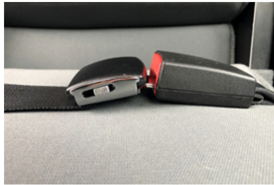
Parallel/flat and in line with webbing
